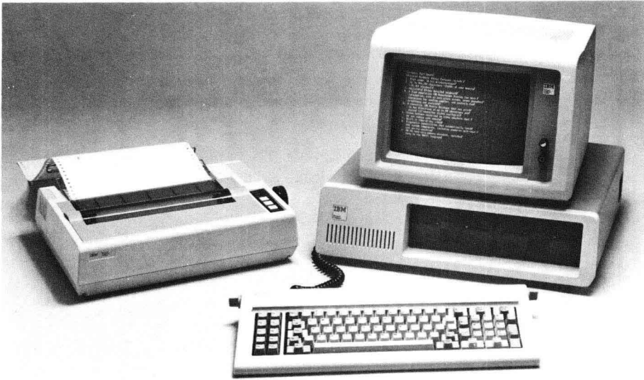
Figure 1.1 An IBM Personal Computer. The keyboard unit and the video display are easily recognized. The video display is atop the system unit, to the left of which is the line printer. The black area on the front of the system unit contains two diskette drives.
