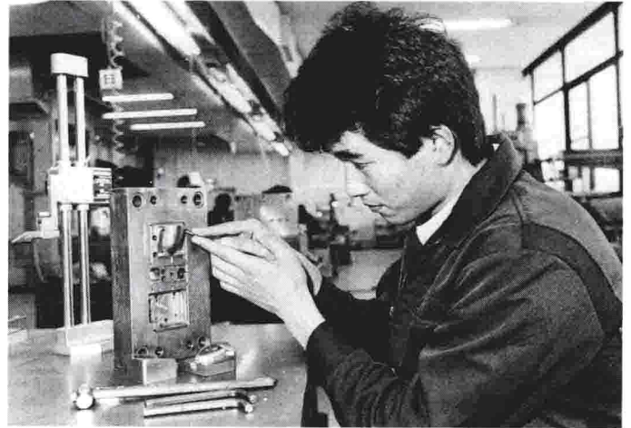
Fig. 1-12. This die for molding plastic model cars started as a block of metal. Metalworking technology, along with human skills and creativity, have converted the metal block into a precisely made tool to produce a product for the hobbyist. (MRC/Tamiya)
