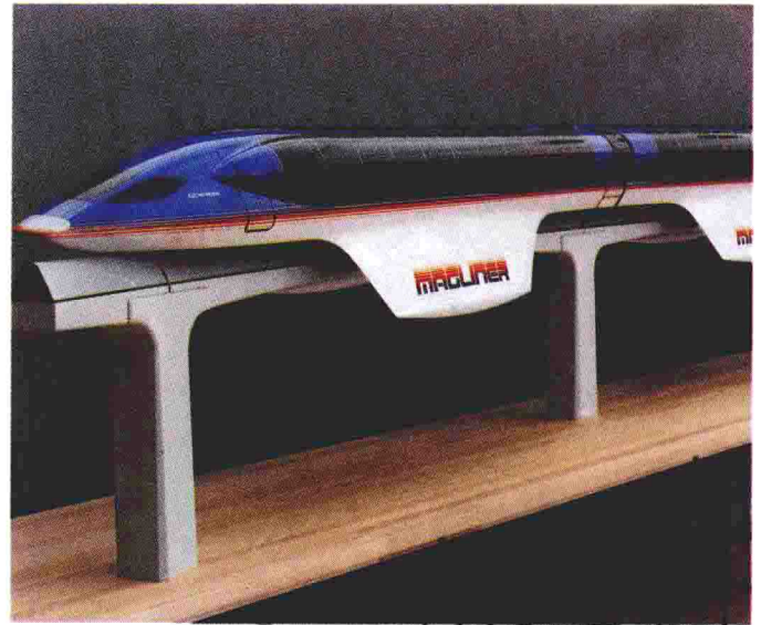
Fig. 1-10. Model of a proposed train of the future called Mag-Lev. Fast, quiet and resistant to derailling, the magnetically levitated train will travel at over 300 miles per hour. It will use super-conductors (transmits huge currents without electrical resistance, and thus sustains intense, steady magnetic fields) to levitate, guide, and propel the train. (Electromotive Division, General Motors Corp.)
