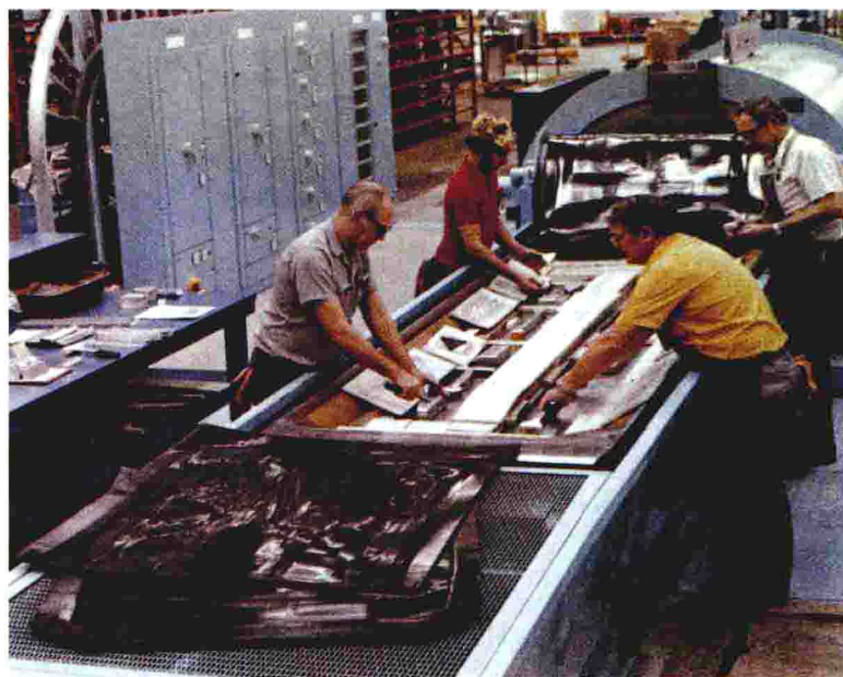
Fig. 1-18. Semiskilled workers perform a limited number of assembly or forming operations, such as shaping aluminum skin fuselage sections for the F-16. They will perform these operations over and over, as long as the aircraft is in production. (General Dynamics)
