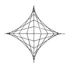
astroid. It is possible to construct this curve in the following way: make a circle of diameter d/2 roll inside another circle of diameter 2d and draw the trajectory of any particular point of the rolling circle. This trajectory will be the astroid. We shall discuss this curve and its close relatives in Sec. 7 of our book where the reader will make a more detailed acquaintance with the interconnection between the problems which we have discussed.
