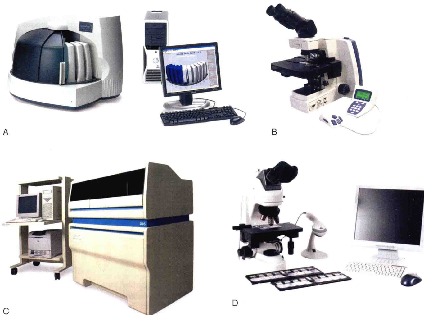
Figure 1.2 Automated cytology screening devices. A, ThinPrep Imaging System: the imager. The imager consists of (left to right): the imaging station, an image processor and server, and a user interface consisting of a monitor, keyboard, and mouse. B, ThinPrep Imaging System: the Review Scope. Imaging data are electronically linked to a customized microscope called the Review Scope. After the ThinPrep slides have been imaged, they are brought to the RS for location-guided review. In addition to a microscope, there is a console (with display and keypad) and a navigator pod. C, BD FocalPoint Slide Profiler. The FocalPoint Slide Profiler consists of two main components (left to right): the workstation (computer, monitor, keyboard, mouse, modem, and printer) and the floor-standing instrument (slide processor). D, BD FocalPoint Guided Screening Review Station. After SurePath slides have been imaged, they are brought to the Review Station for location-guided review. Imaging data are electronically linked to a customized microscope. In addition to the microscope, there is a barcode scanner and a monitor with keyboard and mouse. (A and B courtesy Hologic, Inc. and affiliates. C and D courtesy BD Diagnostics Inc.)
