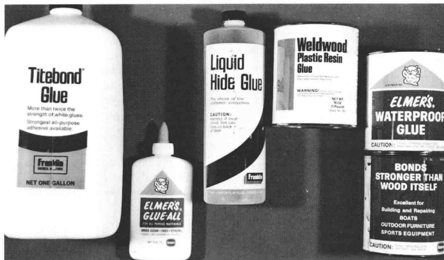
Fig. 1-7. All of these glues are satisfactory for bonding of woods and other furniture materials.
