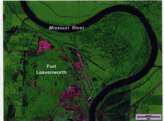
Plate 3-17. Ikonos false-color composite of Fort Leavenworth, northeastern Kansas, United States. Green, near-infrared and red bands color coded as blue, green and red; active vegetation appears dark green to yellow-green colors. Dataset acquired August 2000; compare with Figure 3-16. Image from NASA; processing by J.S. Aber.
