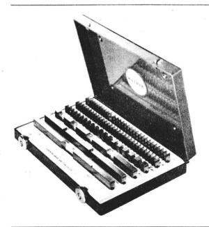
Fig. 1.4 Metric slip gauges.
