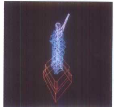
FIGURE 14-16 The Statue of Liberty's interior skeleton counteracts forces and torques acting on the statue. Computer-drawn images of Liberty's skeleton helped engineers and architects plan its renovation.
