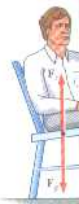
FIGURE 5-15 The gravitational force F_g on a person causes downward acceleration. If the net force must be zero, it is the upward contact force F_c provided by the chair seat.
