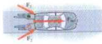
FIGURE 5-13 When two people push a stalled car, the force they exert is the vector sum of their individual forces.
