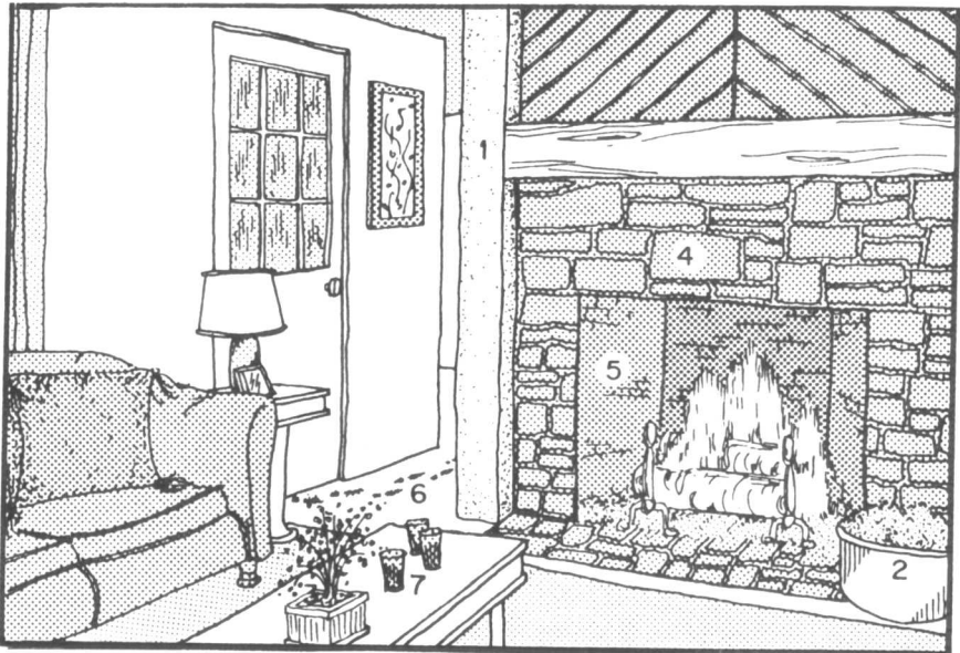
Figure 2.2 Radon, a radioactive byproduct found in concrete (1), sand (2), gravel (3), stone (4), brick (5), soil (6), and drinking water (7), may become confined within a closed house and concentrated to levels up to 10 times higher than those outdoors.
