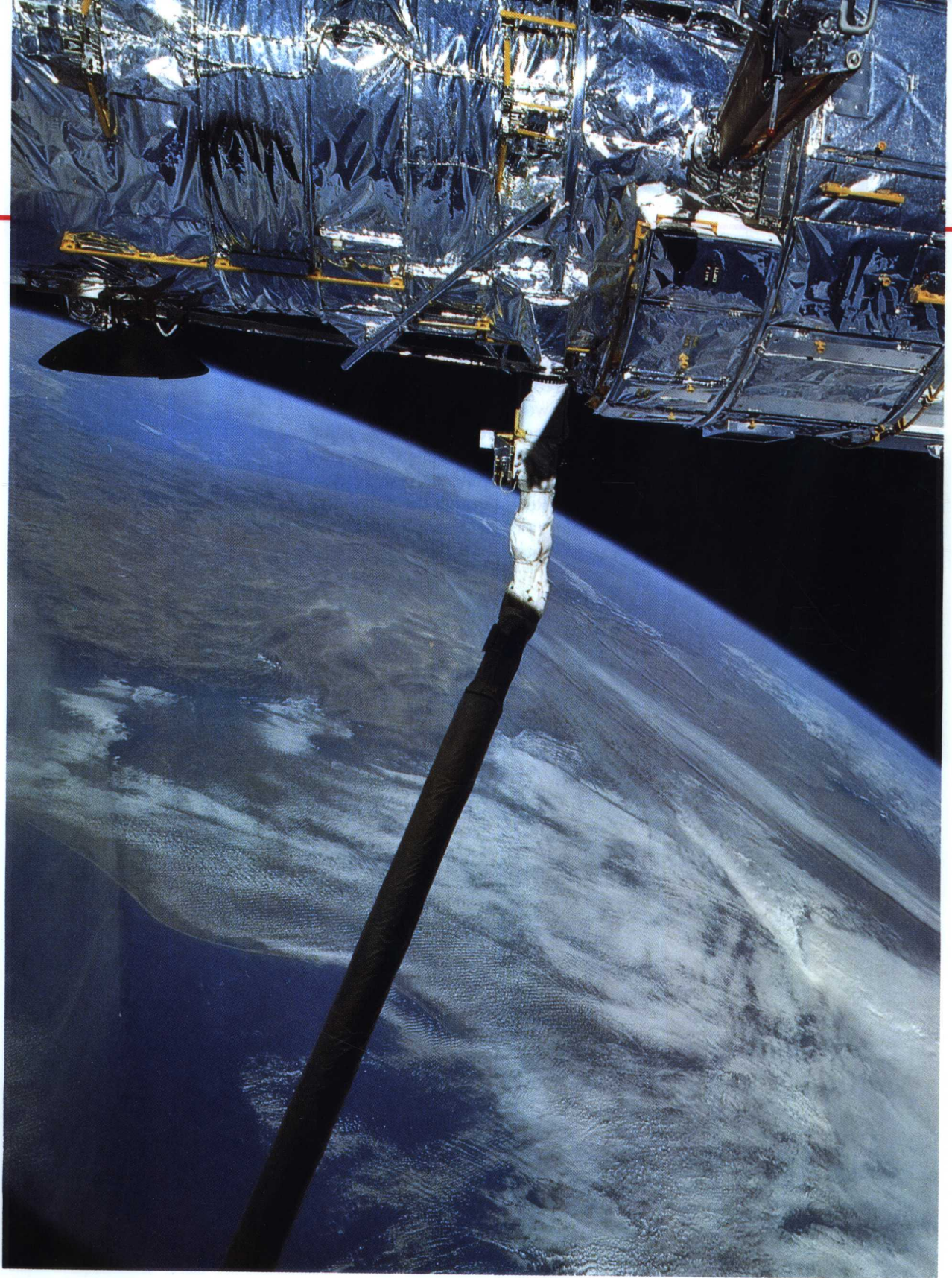
Discovery's remote manipulator system hoists the Hubble Space Telescope (HST) over the Earth's horizon prior to deployment of HST's solar panels and antennae.
