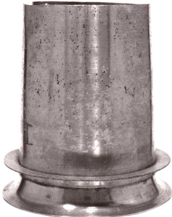
Figure 4. Pitting from the outside of a detail in stainless steel grade 17-12-2.5, which was exposed to a hot, concentrated sodium chloride solution.
