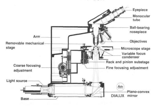
Figure 1-1 Typical working parts of the optical microscope. (Courtesy E. Leitz, Inc., Rockleigh, N.J.)
