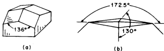
Fig. 2. (a) Vickers and (b) Knoop hardness indenters.
