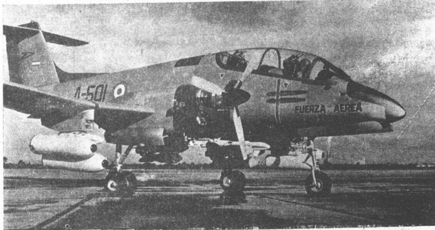
FMA IA 58 Pucará counter-insurgency aircraft for the Argentine Air Force, equipped with underwing and underfuselage weapons
