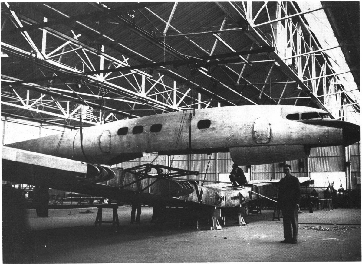
Fig. 1.1 A 1937 venture into composite construction. The de Havilland DH91 Albatross airliner was moulded as a ply-balsa-ply sandwich, carapace construction, upon a male mould. The photograph shows the completed fuselage being mated to the wing. A similar technique was used in the Mosquito to achieve the superb aerodynamic form apparent in both aircraft. British Aerospace plc Hatfield
