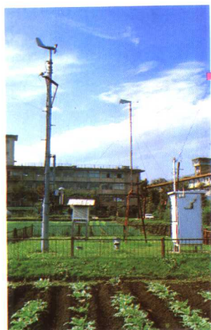
▲ Automatic Weather Station There are 1,313 of these stations nationwide. Each automatically sends data to the computer in the Meteorological Agency. Collection of data from all stations takes only 10 minutes.
