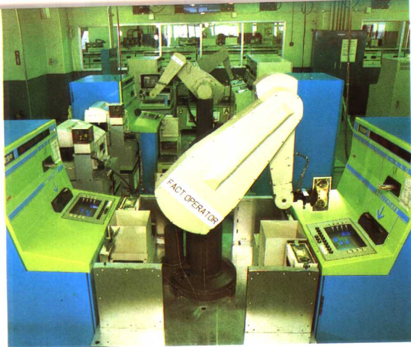
▲ Robot Examiner Computer-controlled robots test the A.T.M.(Automatic Teller Machine). They work 24 hours a day and perform four times as much work as a man does.
