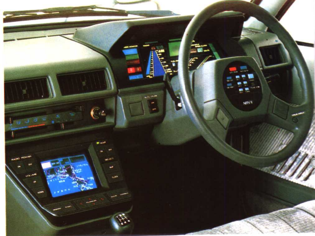
▲ Computer-controlled Car Pre-programmed with the route, the computer responds to oral commands, shows the way, warns and questions by voice when necessary.
