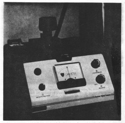
Figure 1-3. Simple dual-beam oximeter for estimation of oxygen saturation.
