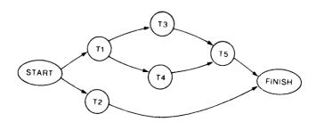
This example chart shows that in the beginning tasks T1 and T2 can both be started. After T1 is done, T3 and T4 can be started, and when both of them are done, T5 can be started. The whole project is finished when T2 and T5 are done. As the next example will show, precedence charts can be used to specify concurrency in computer programs.
