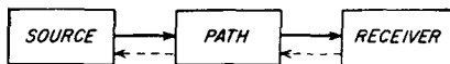
FIG. 1.1. Schematic diagram in which the heavy solid arrows represent the transmission of sound from a source to a listener. The block labeled source may represent more than one sound source; the paths may be numerous; and the receiver may represent a single person, a group of people, an entire community, or equipment whose operation is affected by noise. The broken arrows indicate interaction between the various elements of the block diagram.
