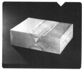
60 mm plate AlMg5, X joint welded in 2 x 2 layers, 3.2 mm ø wire. Root passes: plasma 250A, MIG 440A, wire speed 7 m/min, welding speed 27 cm/min. Filler passes: plasma 220A, MIG 320A, wire speed 4.5 m/min, welding speed 10 cm/min. Torch oscillation ~ 1.5 Hz.
