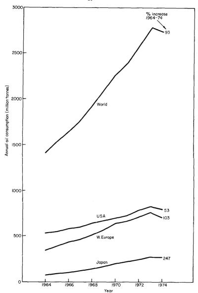
1/2 Oil consumption, 1964-74. An indication of the need for energy conservation, and of the effect on consumption of a recession in world industrial activity.
