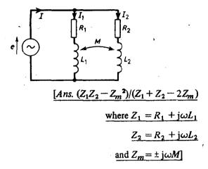
16. Experiments carried out on a variometer, whose two coils were series-connected, showed that the inductance values obtainable varied from 40 mH to 360 mH. Assuming that the self-inductances of the two coils are equal, determine the range of inductance values obtainable if the coils are reconnected in parallel. Neglect resistances.
