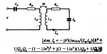
9. Two series circuits, each consisting of a 300- $\mu$ H inductor and a 1069- $\mu\mu$ F capacitor, are magnetically coupled so as to have a mutual inductance of  $60\mu$ H. A voltage of 10 V having a frequency of  $1/\pi$  MHz is injected into one circuit. Determine the current in the other circuit and the coefficient of coupling (k).
