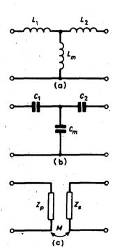
8. The two resonant circuits shown are tuned to the same frequency  $\omega_r/2\pi$  and coupled together. Obtain an expression for the secondary current  $I_s$  in terms of the voltage V, the circuit Q's,  $Q_p$  and  $Q_s$ , the coefficient of coupling k and the ratio of the actual frequency to the resonant frequency,  $\alpha$ .
