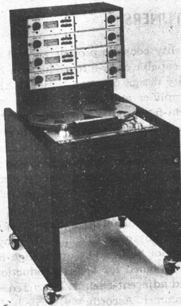
FIG. 1-6. A professional quality reel-to-reel tape deck. (Courtesy of Ampex)
