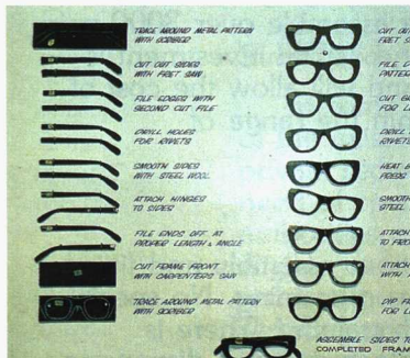
Making spectacle frames — sheet plastic method
