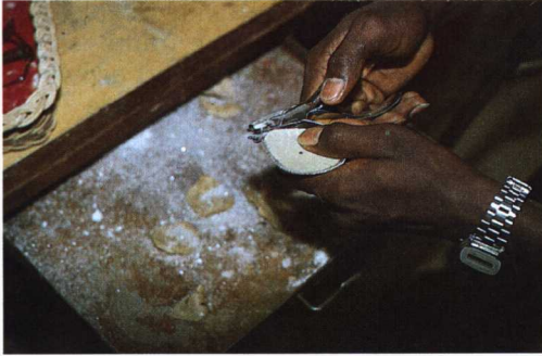
The cutting and shaping of lenses in a small optical workshop
