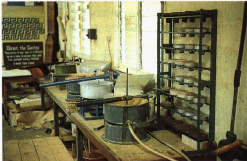
The polishing of lenses can be achieved with simple machinery which can be produced locally (see also page 16)
