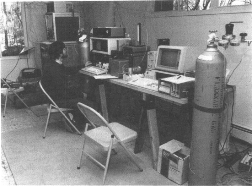
FIG. 1—The array of airflow measurement systems in the living room of the basement test apartment. From left to right are the multiple tracer measurement system (MTMS), the constant concentration tracer gas (CCTG), and the “real time” version of the perfluorocarbon tracer (PFT). Two other versions of the PFT systems are not shown.
