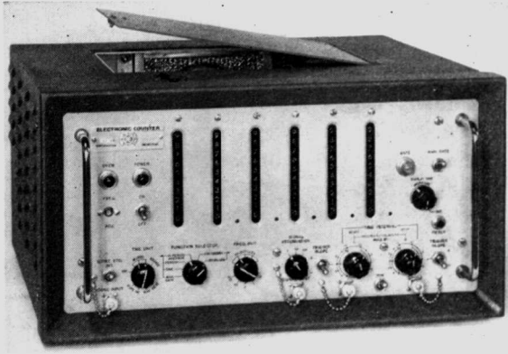
Fig. 1-2 Counter used to measure units of time, to count events or electric pulses, and to measure frequency. (Northeastern Engineering)
