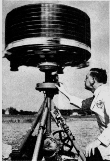
Fig. 1·1 Solar cells used to generate electric current directly from the sun's rays on Tiros satellite. ( International Rectifier Corporation )
