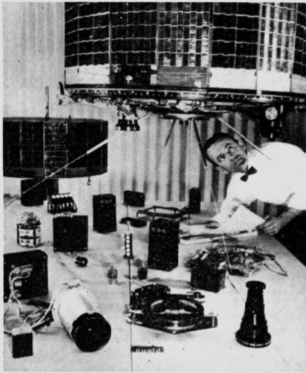
Fig. 1·1 Solar cells used to generate electric current directly from the sun's rays on Tiros satellite. ( International Rectifier Corporation )
