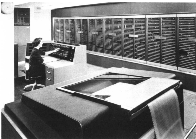
Figure 1.2. The most powerful computer in the mid-1950s was the Naval Ordnance Research Calculator. It contained 9,000 vacuum tubes. (Courtesy of IBM Corp., White Plains, New York.)
