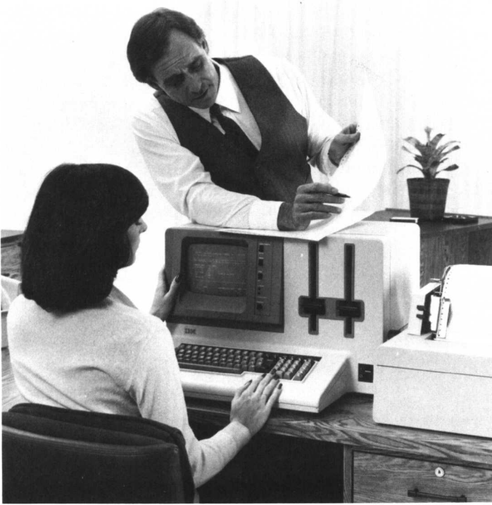
Figure 1.5. The IBM Model 5120 desktop computer has the power of equipment that 20 years ago filled a 20-by-30-foot room and weighed a ton. (Courtesy of IBM Corp., White Plains, New York.)
