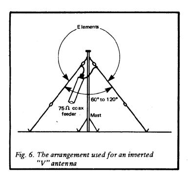
available or are easily improvised. For example, aerials of this type are often installed over the pointed roof of a house (but must be kept reasonably well clear of the roof in order to obtain good results).
