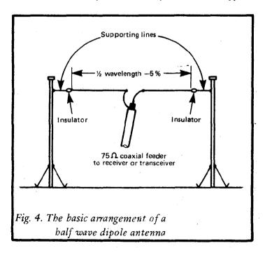
in the usual way using insulators, and lines made from an insulating material between the elements and the masts or other supports.
