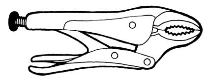
Locking pliers Locking pliers provide an adjustable, viselike grip that, once in place, holds a fitting by itself.
