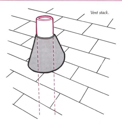
Vent stacks are pipes that protrude through the roof from the waste lines. They equalize the air pressure in the drain system and prevent the suction generated by flowing water from siphoning the water out of the traps and commodes.
