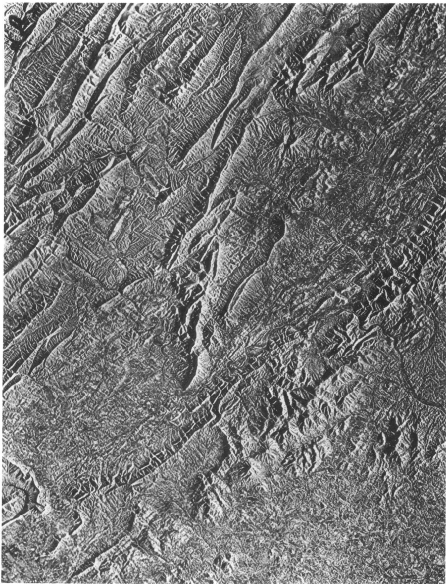
Figure 1-3a Side-looking radar image of a portion of the Blue Ridge and Valley and Ridge provinces in the Central Appalachian Mountains. Rock structure shows up because rocks that are resistant to weathering and erosion have been etched out. ( U.S. Geological Survey Image. )
