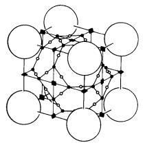
Fig. 1 Unit cell of cubic  $\alpha$ -AgI.
