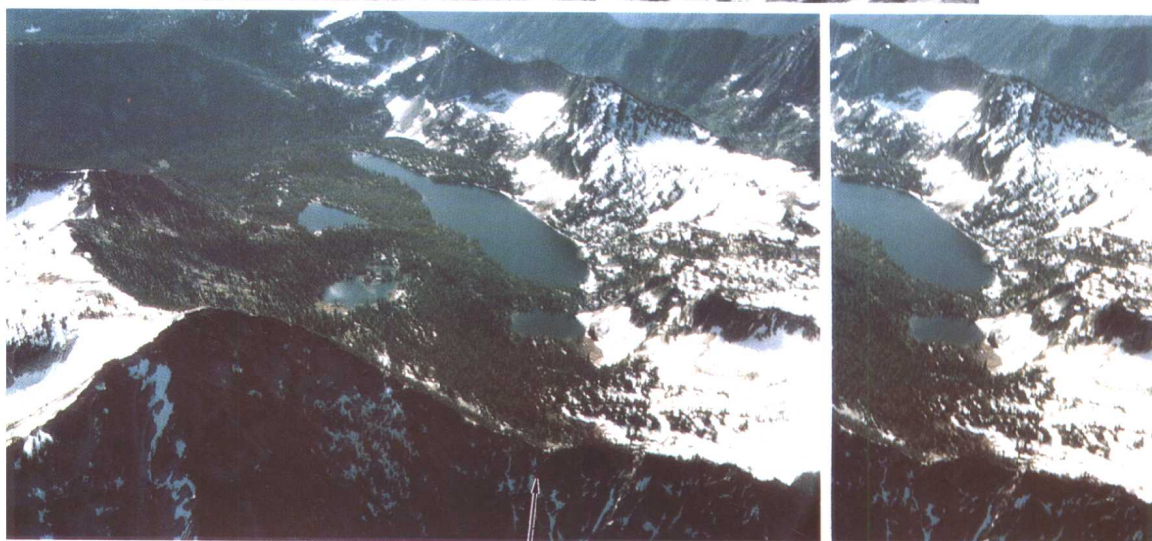
Top: Radar imagery of the Enos Lake Quadrangle and environs of Idaho's Payette National Forest, acquired from an altitude of 60,000 feet with the AN/APQ 97 side-looking airborne radar (SLAR) system. Note the accentuation of terrain features in this highly glaciated topography. Bottom: A low-altitude aerial oblique stereogram that was taken (as indicated by matching arrows on the top and bottom figures) while looking through the notch between North Loon Mountain and South Loon Mountain. Note that while some features are better seen on this low-altitude stereogram, others are better seen on the very high altitude radar imagery. (Courtesy of NASA and the Nationwide Forestry Applications Program of the U.S. Forest Service).
