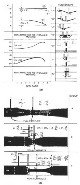
Figure 1-2. (a) Shows discharge coefficient's dependence on beta ratio. (b) Schematic of flow mechanisms.
