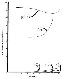
Figure 1-4. Relationship between kinetic energy and beta ratio.
