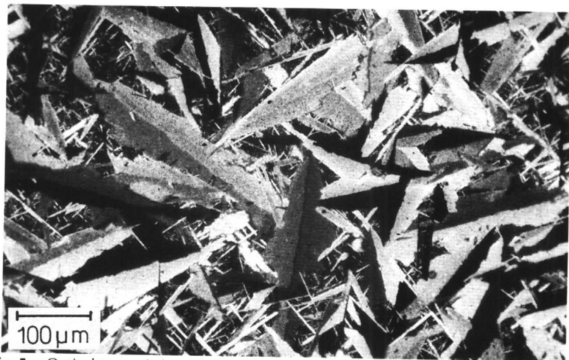
Fig. 5. Optical transmission micrograph of silicon carbide specimen doped with boron and carbon.
