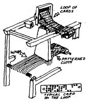
in ordinary loom is special-purpose. It can weave cloth only in the usual underand-over kind of way. A Jacquard loom is different. It has a loop of cards with holes punched in them. Each card in turn comes against a set of needles. Wherever there is a hole in the card a needle falls through—and this causes a corresponding thread of the warp to be lifted. The pattern of holes in the loop of cards thus determines the pattern on the
