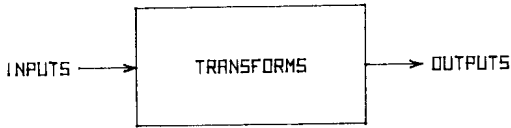
Figure 1.1. General system theory view of relationships among inputs, transforms, and outputs.
