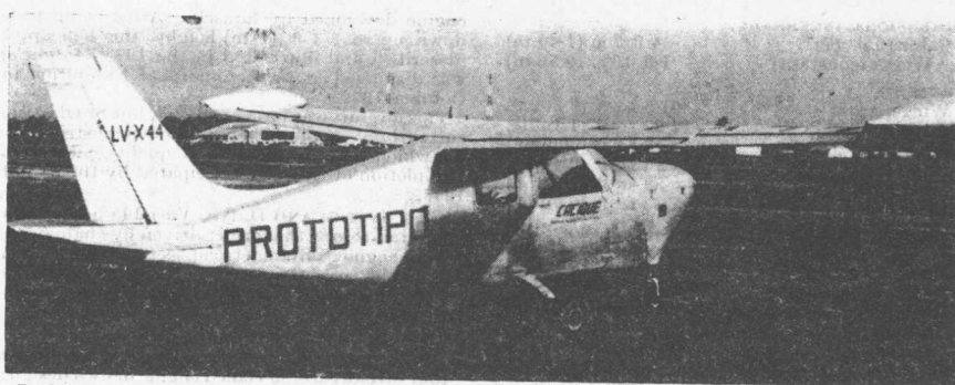
Prototype Turbay T-11 Cacique light aircraft (100 hp Continental O-200-A engine) (Alex Reinhard)
