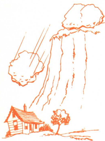
Figure 1.8 A boulder on a cliff represents potential energy. A falling boulder represents kinetic energy. The falling boulder can do work (smash a house, for example). The boulder on the cliff has a potential for doing the same thing.
