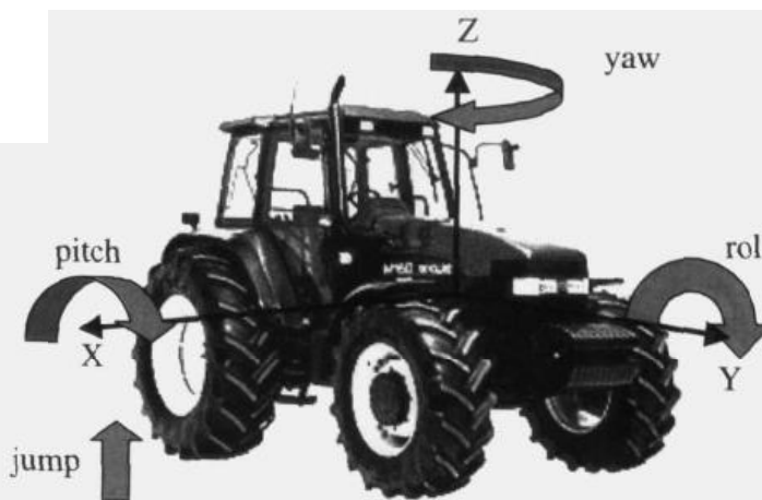
Figure 9. Explanation of the mode shapes roll, pitch, yaw, and jump.
