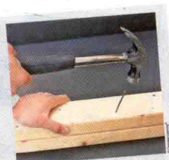
FIGURE 1-41 Stagger nails for greater strength and to avoid splitting the stock.
