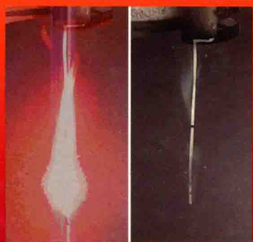
UL94 test: without and with flame retardant
