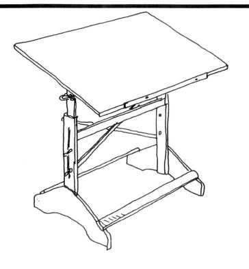
A sturdy drafting board, either a lap or table type, is necessary for serious drafting. A metal edge is required if a t-square is to be used. The surface should be covered with a drafting cover such as *Borco* plastic for maximum utility. The surface should never be cut on or punctured with tacks. Only drafting tape is acceptable for fastening drawings. The board should be larger than the largest sheet of paper you expect to use. A typical board size for interior design drawing is 30" x 42".
