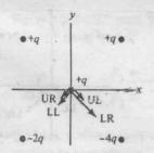
Coulomb's law can be used to calculate (for example) the force UL by ignoring the other-three charges.
