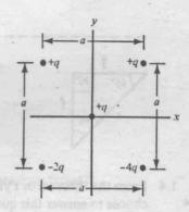
1.1 The approach to this problem invokes the principle of superposition. Superposition means that we can calculate the total force on the charge at the center by first pairing the central charge q with each of the four surrounding charges and then determining the vector sum of the four forces.
