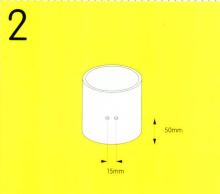
\_Drill two 6mm holes on one of the short pieces of pipe.
