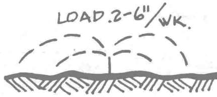
Figure 1-1 Surface irrigation. Load is sprayed in 4-8 hr (2 in./week at Pennsylvania State Project; 4 in./week at Muskegon Project).
