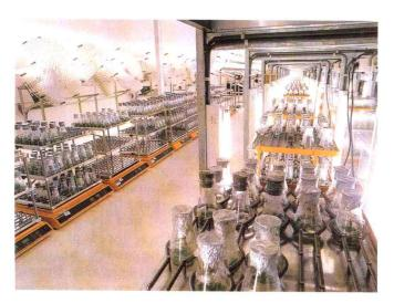
Figure 2.3. Shakers for the aeration of liquid cultures. (By P+S PLANTLAB b.v., The Netherlands)
