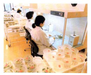
Fig. 2.1. Laminar flow hoods for aseptic procedures. (By Van Staaveren bv, Rijsenhout, The Netherlands)
