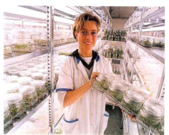
Figure 2.2. A walk-in controlled environment room for incubation of *in vitro* cultures. (By SBW, Rijsenhout Department, The Netherlands)
