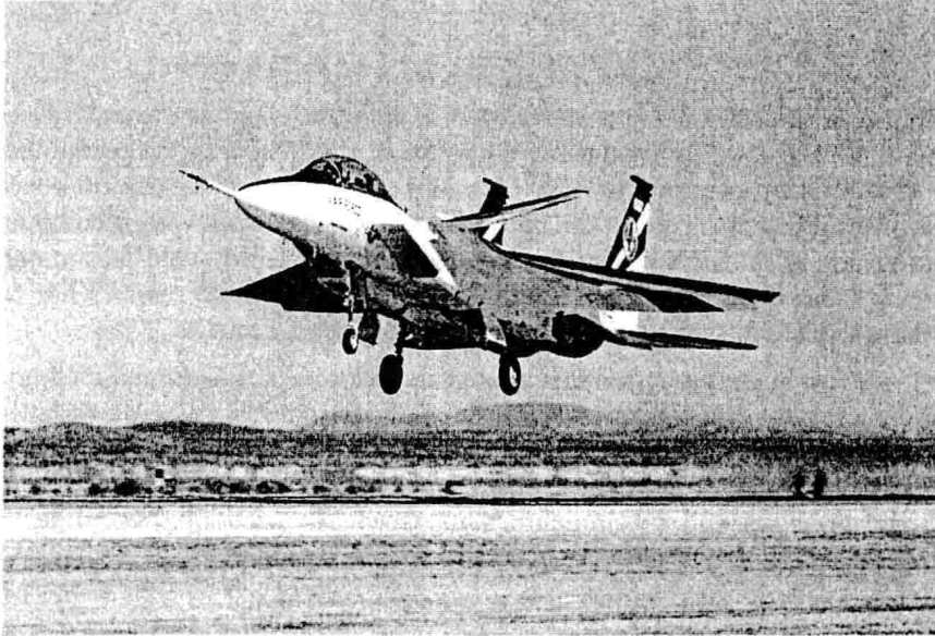
Figure 1.1. The NF-15B research aircraft. Boeing and the NeuroEngineering Group at NASA Ames Research Center have developed an adaptive neural-network-based flight control system capable of recovering from damages due to failures or serious accidents. The control system has been tested on the NF-15B at NASA Dryden Flight Research Center. The F-15 has been modified so that damages can be simulated by activating the canards (the small front wings), thereby changing the airflow over the main wings. (NASA Photo by Tony Landis, Dryden Flight Research Center.)
