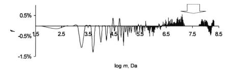
Figure 2. GMS spectrum of a dried evergreen laurel leaf (see Figure 1),  $p < 1 \text{N/m}^2$ , Zubow constant is equal to  $6.4 \cdot 10^{-15}$  N/m, N = 708, D<sub>c</sub> = 42 % and M<sub>GMS</sub>= 92,518,741 Da.
