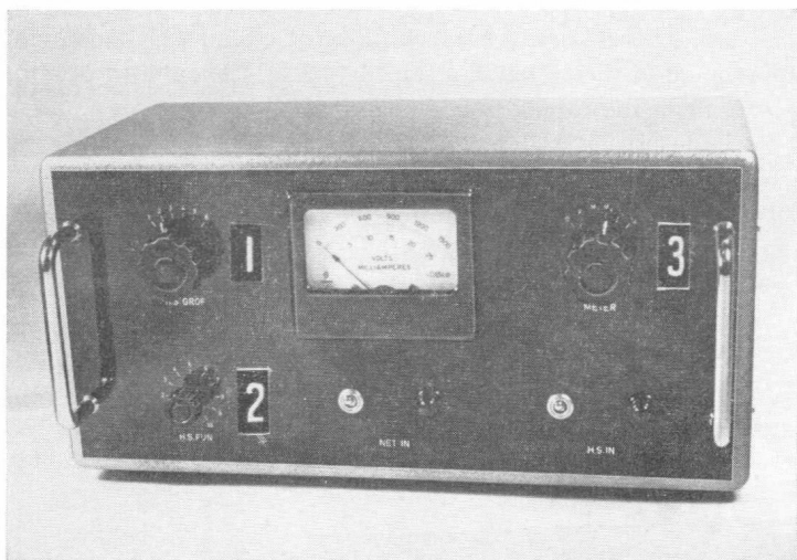
Fig. 2. Power pack for zone electrophoresis (constructed by Mr. W. L. van Es of the Physical Department of the Netherlands Cancer Institute); constant voltage from 0-1,500 V, maximum current 25 mA. 1 = Voltage range switch (coarse), 2 = Voltage range switch (fine), 3 = Switch for monitoring system: O = off, V = output voltage, M 1 = voltage on the column, M 2 = voltage on the 2nd column, I 1 = current, I 2 = current through the 2nd column.
