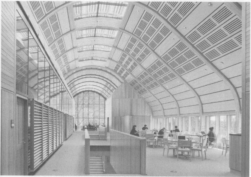
Figure P.2 The daylighted top-floor reading room and café at Kroon Hall, Yale University. Photovoltaic panels over skylights generate energy and filter the sun, which balances sidelight seeping through the building's protective exterior louvers. Credit: © Robert Benson
